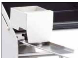
The clips storage (optional) always keeps clips to hand for sealing the bread bags.
