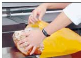
The bagging aid allows even long loaves to be bagged easily.
