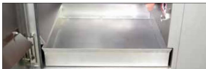
An easily removable tray successfully catches all the crumbs. This is assisted by guide plates etc. The crumb tray can be emptied and brushed out in no time. Bread cannot be sliced more hygienically than this.
