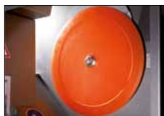
The Teflon-coated blade has unique tothing and a special grinding finish. Combined with planetary gearing, these features allow fresh bread to be sliced without blade lubrication.
