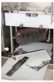
Blade set conveniently pivots outward when disassembling to ensure quick, complete and easy sanitation
