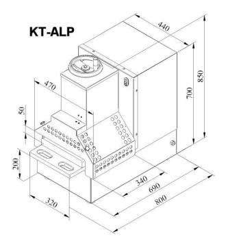
Dimensions: (w/out stand) 32.09" H x 19.69" W x 28.74" D Motor: 2hp Machine Weight: 385 lbs Voltage Requirements: 220v/3 phase
